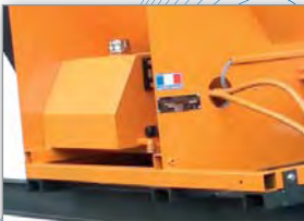
Hydraulic tank and distributor unit
