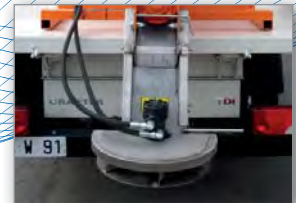
Rear spray unit all stainless steel
